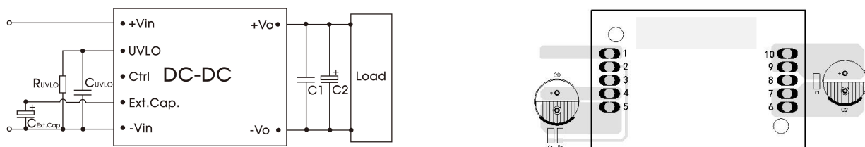
Fig.7 Recommended circuit and PCB layout for hold-up time
