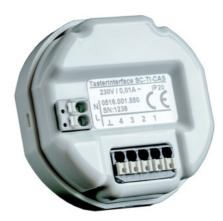
The SC-TI-CAS is an input module for up to 4 potential-free buttons. The device is automatically recognized by the Casambi app and can be included in the existing network. The functions triggered by the buttons can be configured with the Casambi app.
